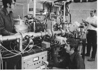
DISCUSSING OBJECTIVES OF NEXT ION-IMPLANTATION EXPERIMENT in Diffusion Properties Lab are (I to r) Wayne Chrisman, Dan Morse and Walt Bauer (all 8331). Analysis of samples without removing them from the accelerator's target chamber (located in front of Bauer) is unique feature of Sandiadesigned chamber and mass spectrometer. Lab is studying the mechanism of inert aas migration in metals and alkali-halides.
